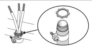
Fit a squeeze connector (not supplied with the range), to your conduit. Insert the conduit through the reducer plates on the mounting bracket. Allow enough slack to easily attach the wires to the terminal block.
